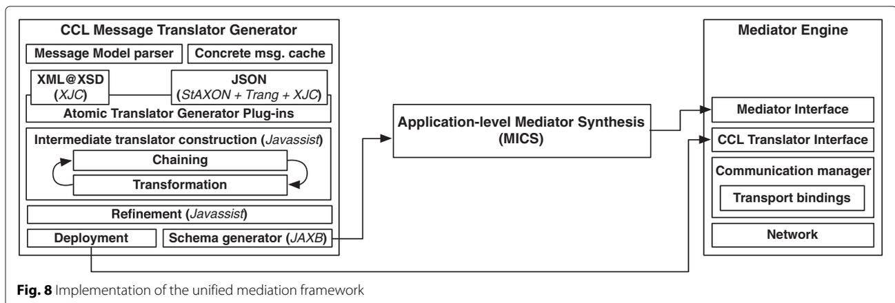
Fig. 8 Implementation of the unified mediation framework
