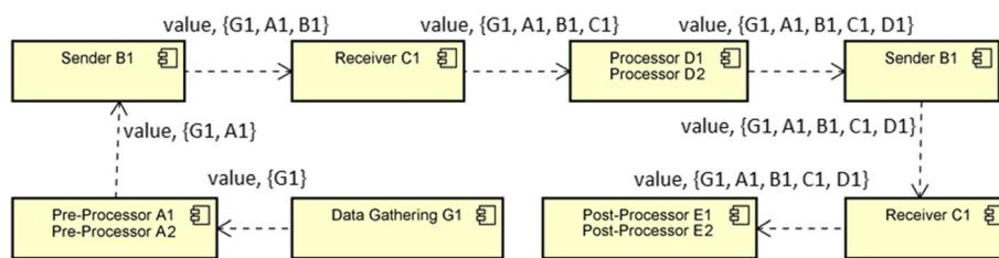
**Fig. 7** Execution path of the data in a partially reconfigured system
