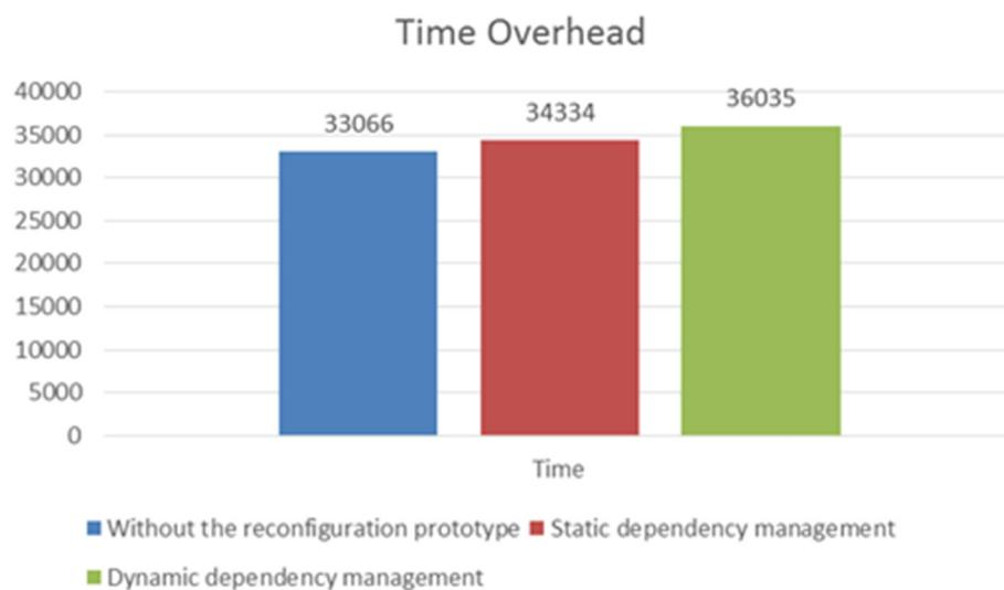
**Fig. 19** Overhead in terms of time imposed by the reconfiguration prototype
