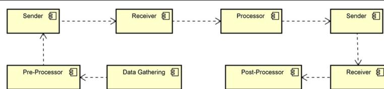
**Fig. 2** Illustrating scenario in which data is gathered and pre-processed before being sent to a distributed node, which is in charge of processing the data
