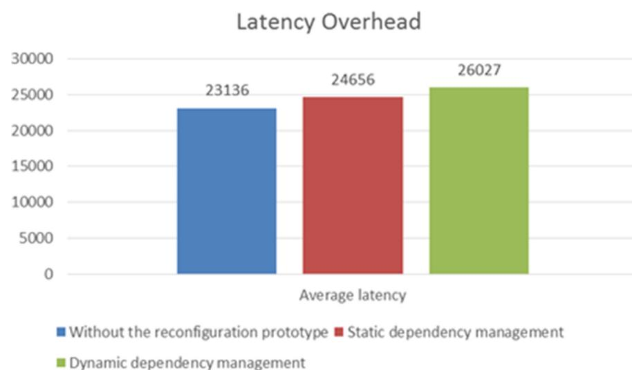
**Fig. 21** Overhead in terms of tuples' latency imposed by the reconfiguration prototype
