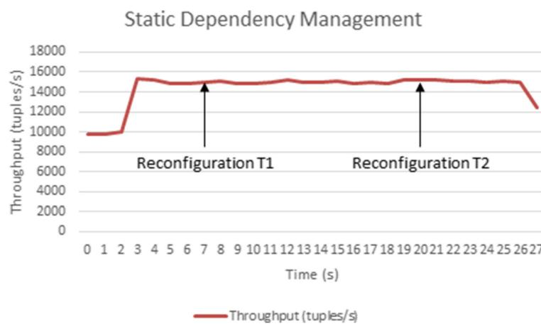
**Fig. 15** Throughput in the scenario with 300 CNs, 15,000 tuples/s and static dependency management
