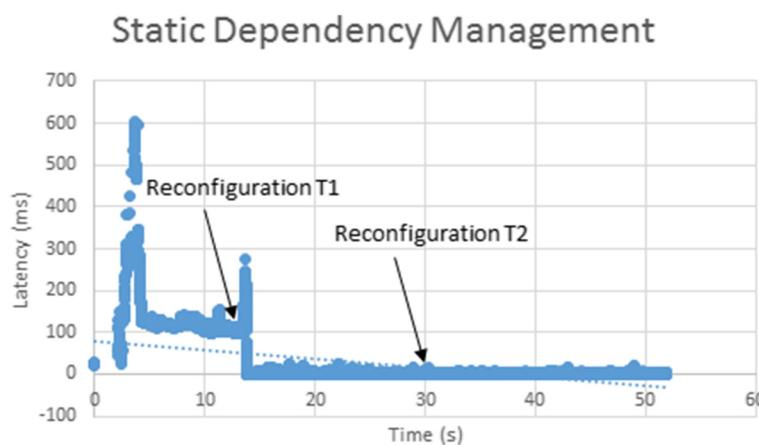
**Fig. 17** Latency in the scenario with 300 CNs, 15,000 tuples/s and static dependency management
