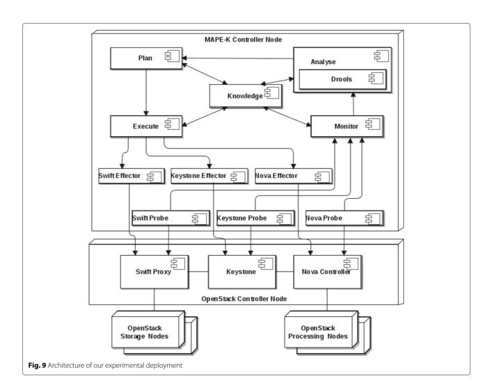
OpenStack Controller Node. The OpenStack Controller Node contains the following OpenStack components: Swift Proxy, Nova Controller and Keystone. Swift Proxy is the component responsible for managing access to the storage service, while Nova Controller takes care of virtual machine management, and Keystone deals with identity management. The MAPE-K controller is hosted in the "MAPE-K Controller Node".
