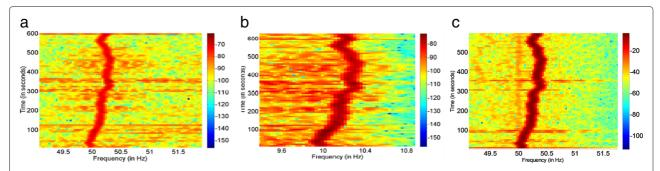
Fig. 6 An example of intrinsic evidence related to the power grid. Showing here are spectrograms of ENF signals in concurrent recordings of a audio, **b** visual, and **c** power main. Cross-correlation study can show the similarity between media and power line reference at different time lags, where a strong peak appears at the temporal alignment of the matching grid
