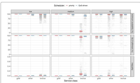
**Fig. 9** Fairness. Confidence intervals of the minimum availability, SLO fulfillment, and inequality of the availabilities of active requests, per service class, in 10-minute intervals with low, medium and high contention for resources
