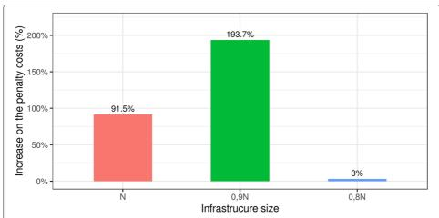
**Fig. 8** Penalty. Increment on the penalty cost when using the priority-based scheduler in comparison to the QoS-driven scheduler
