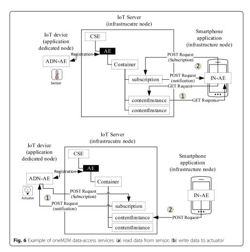
by creating a new <contentInstance> under the container for light control with the HTTP POST Request.
