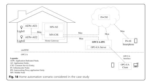
oneM2M service platform IN-CSE. Finally, MN-AE is a gateway application embedded into the home gateway that interacts with the MN-CSE through Mca reference point.
