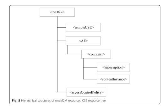
The concept of subscription to resource instances in order to receive notifications about content changes is also specified in oneM2M; it allows efficient monitoring of resource instances and thus of the exposed resources. In particular, the resource defined as <subscription> contains subscription information to a particular resource.
