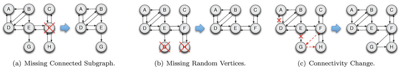
Fig. 2 Examples of anomalies acting on the tiny web graph
