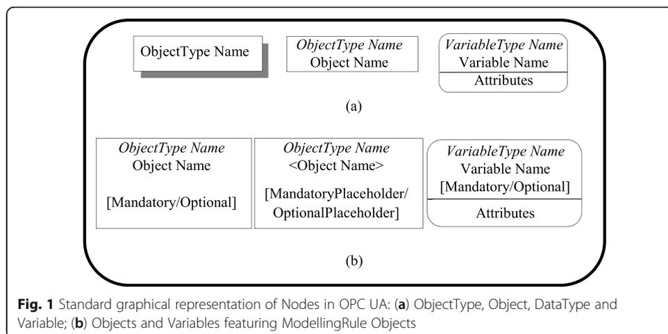
**Fig. 1** Standard graphical representation of Nodes in OPC UA: (a) ObjectType, Object, DataType and Variable; (b) Objects and Variables featuring ModellingRule Objects
