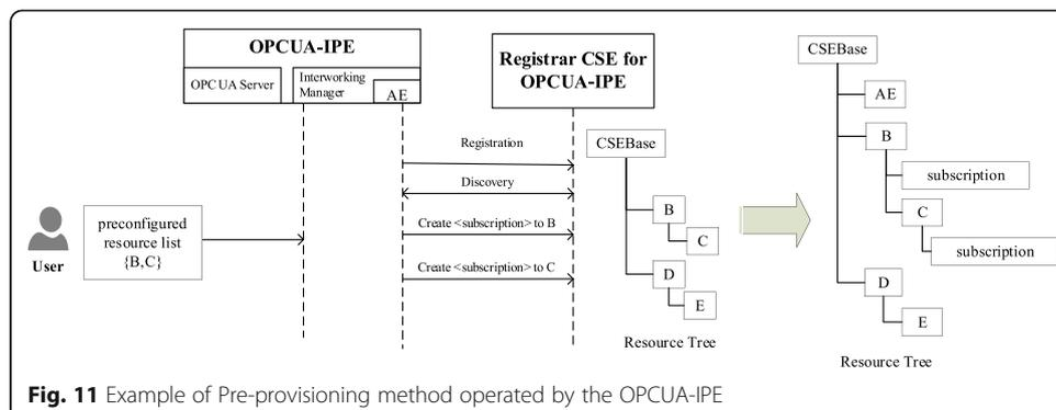
**Fig. 11** Example of Pre-provisioning method operated by the OPCUA-IPE
