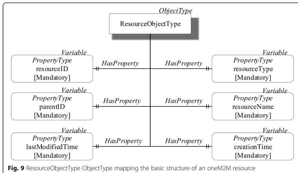
**Fig. 9** ResourceObjectType ObjectType mapping the basic structure of an oneM2M resource
